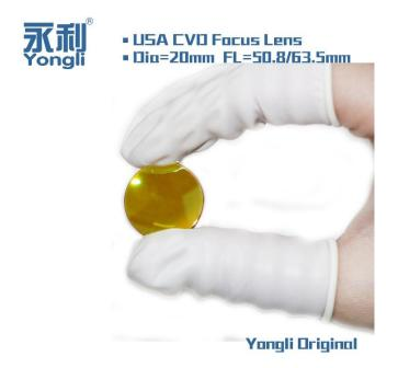
After making sure that the lens is contaminated, blow the lens with a rubber suction bulb until its surface is free of dust. Be careful not to blow directly with your mouth, because most of the air blown out contains oil, water, etc., which will further contaminate the lens. If there is still dirt on the surface of the lens after the rubber suction, we must gently wipe it with a special cotton swab dipped in a mixture of acetone and ether, which will remove most of the
